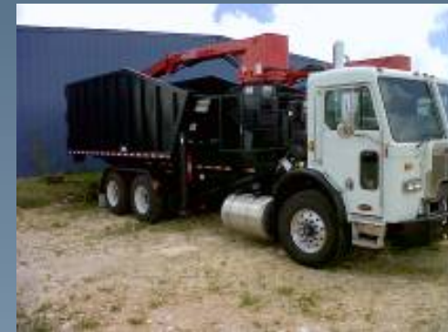
Truck with knuckle-boom grapple hook picks up bulky and metallic waste
